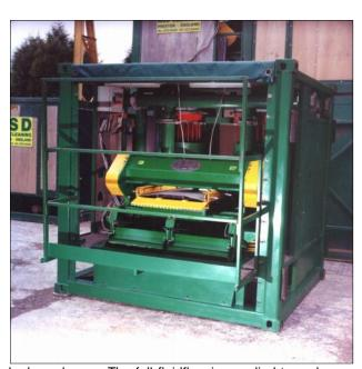
The SU72DP is a compact ultra-fine desilter. The name derives from Supplementary Unit with 72 No. 44mm hydrocyclones and a Discharge Pump. The unit normally works downstream of a desander, a desilter or mud cleaner, but can operate on its own. The machine is used to remove fine sands and silts from low or high viscosity fluids and will separate much smaller sized solids than conventional desilters.
